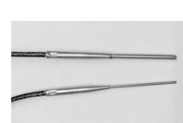
Temperature Probe for rectal temperature measuring. Mouse or Rat.
